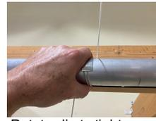
Rotate clip to tighten cord
