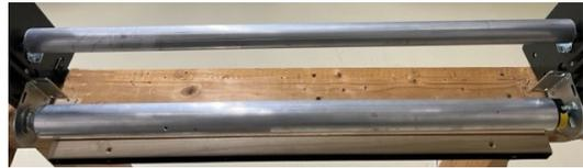
Idler tube on brackets above motor tube.
