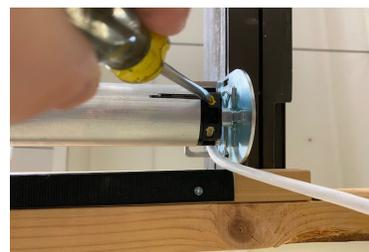
Depress both buttons after removing cap
